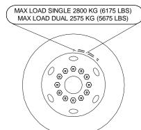
Tire load ratings can be found on the tire sidewall. In the example at left, two of these tires can legally carry 12,350 lbs. on one axle. Four of the tires shown can legally carry 22,700 lbs. on one axle.
